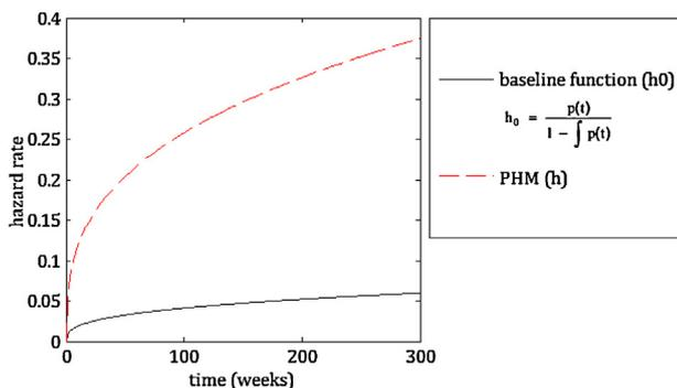
Fig. 5. PHM and baseline hazard rate of generator bearing.
