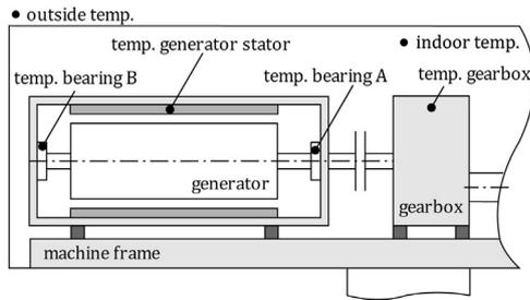
Fig. 4. Wind turbine and temperature measurement spots.
